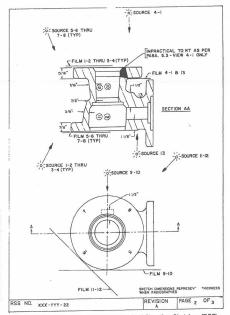
FIG. X1.2 Samples of Radiographic Standard Shooting Sketches (RSS) Views Illustrating Layout and Source and Film Placement
