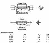
Nore—If desired, the length of the reduced section may be increased to accommodate an extensometer.
